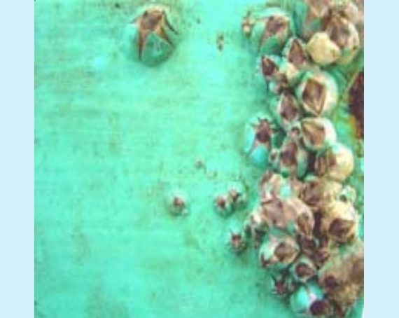
Figure 5c. A dynamic test panel with sufficient erosion of coatings to allow barnacles to attach and push out of the coating. Dynamic test may cause sufficient depletion of the antifoulant to create microscopic damage, which in turn allows barnacles to attach and eventually damage the coating.
