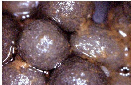
TYPICAL CERAMIC PROPPANTS WITH BACTERIAL BIOFILM
