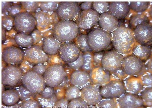
TYPICAL CERAMIC PROPPANTS WITH BACTERIAL BIOFILM
